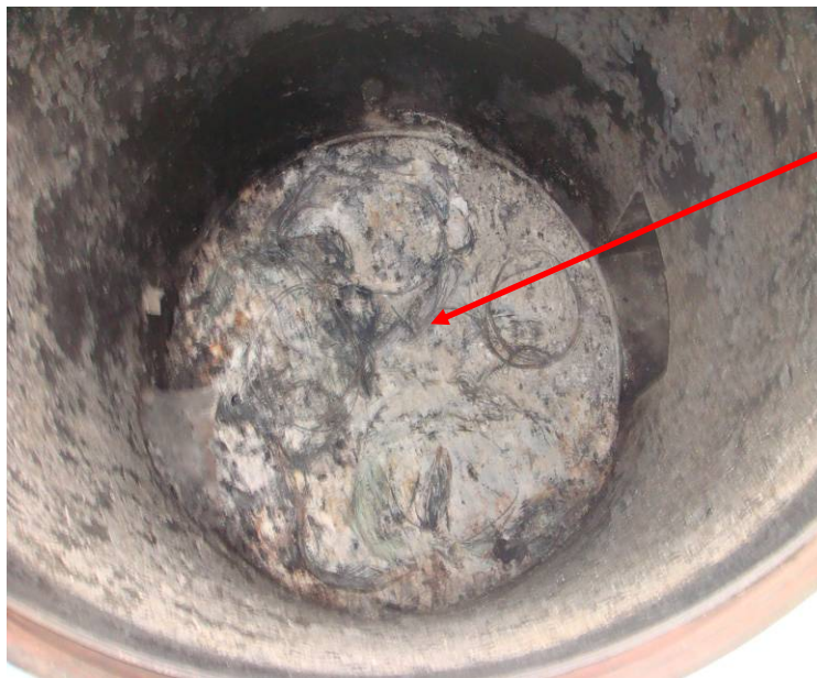
Figure 25: Sample of tire remnants after undergoing the gasification process, which comprises of about 17% tire ash
