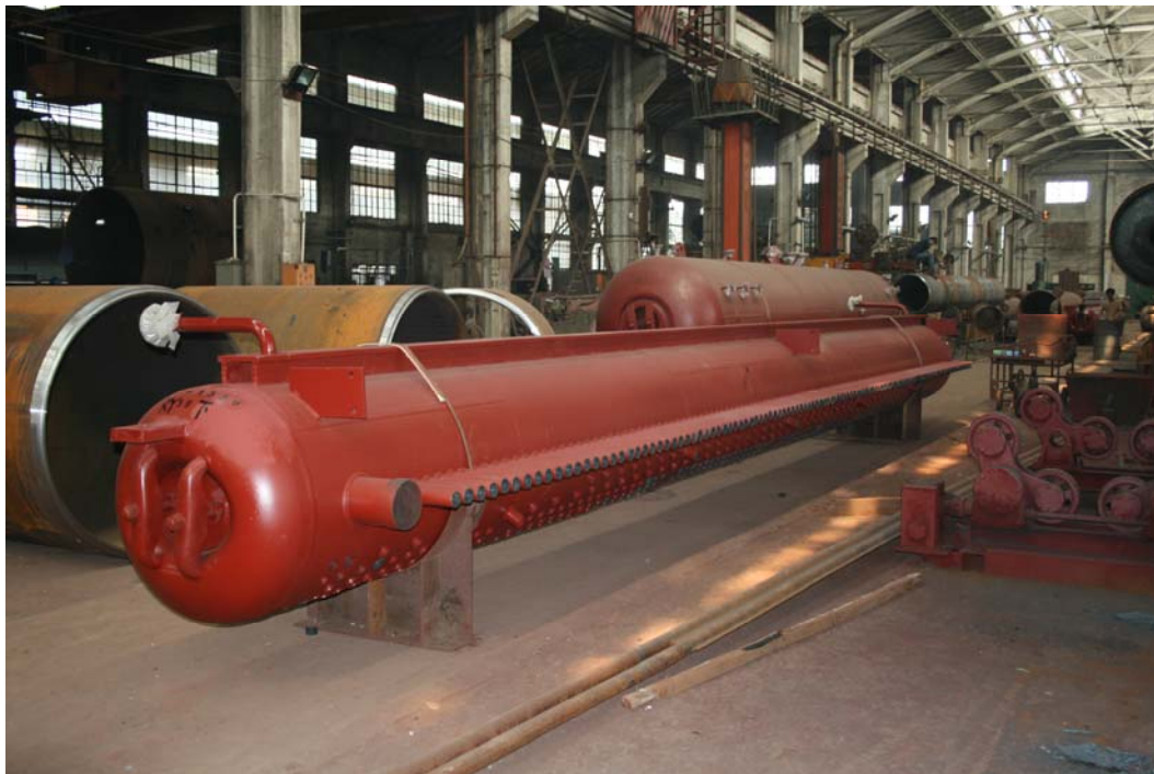
Figure 14: A boiler at the manufacturing plant in SFBW
