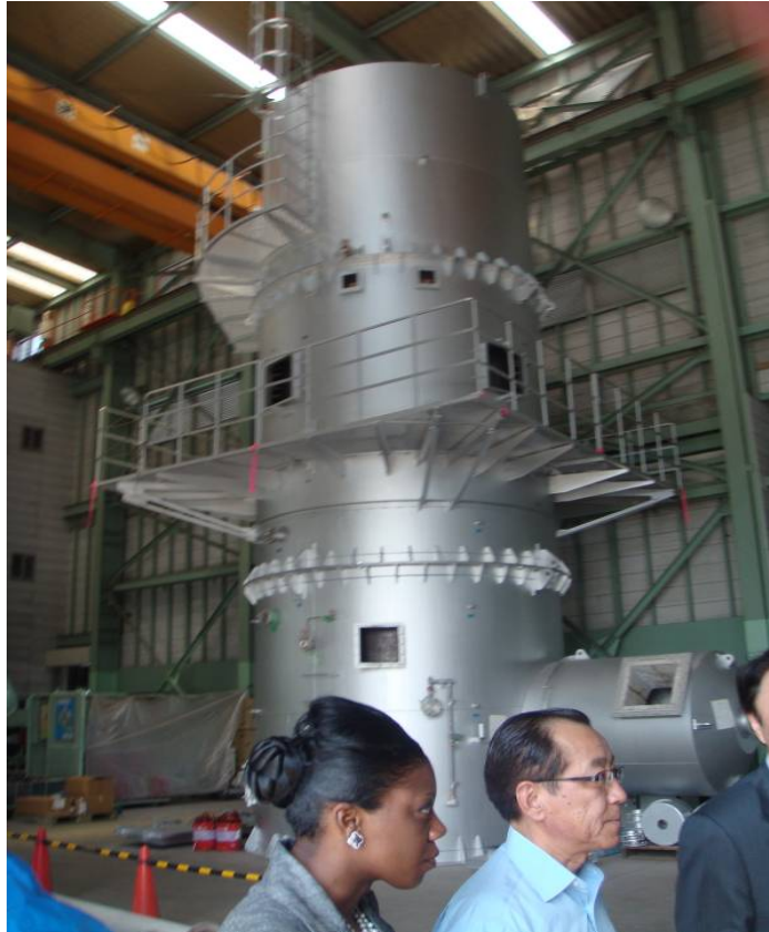
Figure 18: A Kinsei Gasification Plant
