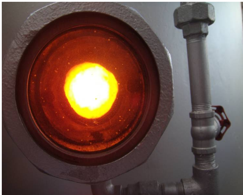
Figure 20: Gasification Chamber under intense heat of about 1200 degrees centigrade and above
