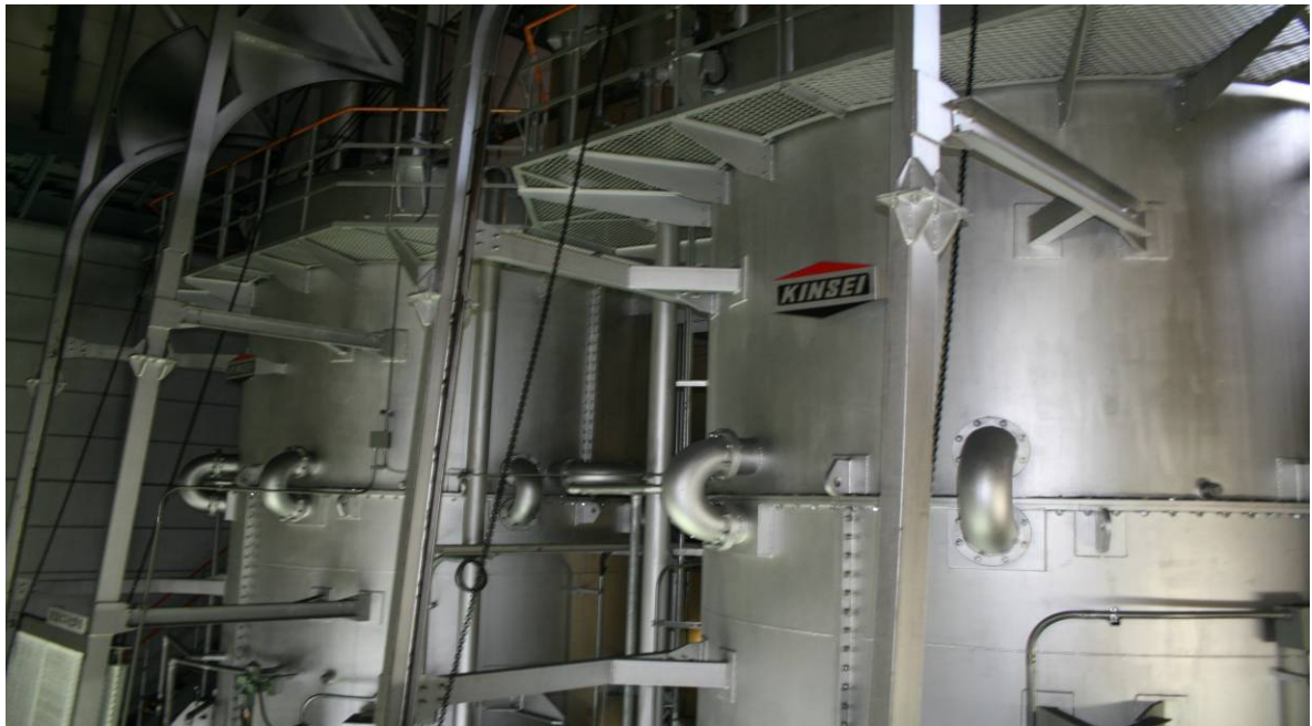
Figure 23: A kinsei gasification system
